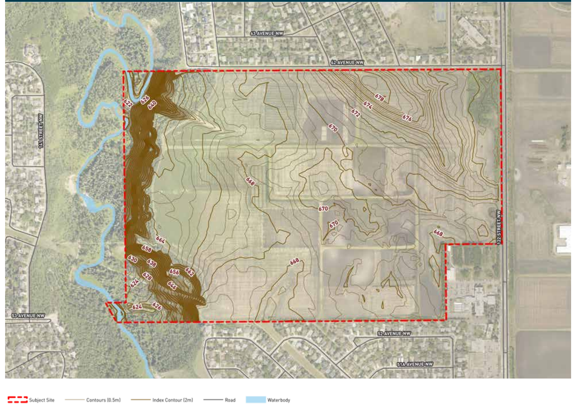
FIGURE 3: Existing Grading & Drainage
